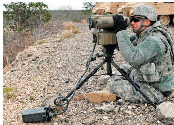
2LT Russel Finegan looks through a Lightweight Laser Designator Rangefinder system during fire support team certification. The LLDR aids Soldiers in determining crucial information during call-for-fire situations while conducting training, or on the battlefield.
