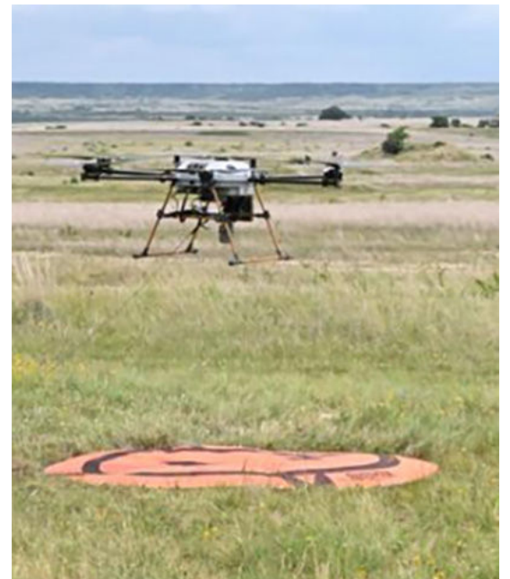
Discovair drone-detection system capable of flying 400 ft in the air prepares for a sensor test flight before the integration demonstration
